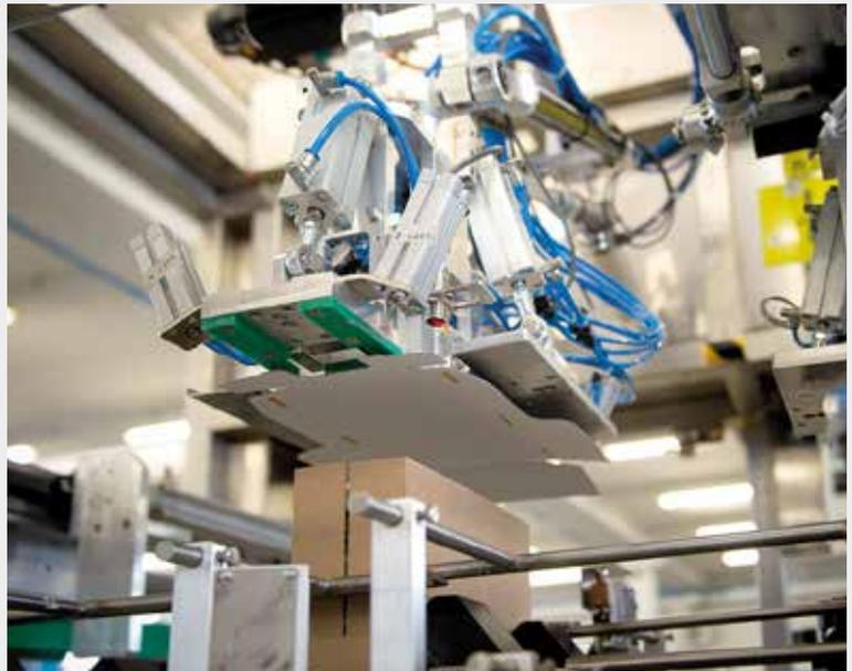
The cartons forming is done with the use of a **pressure matrix** or through **teeth chain** with "U Shape" mechanism in continuous.
